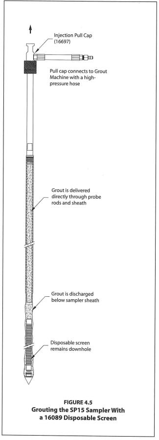
3. Place a mark on the extension rod even with the top of the probe rod. Apply downward pressure on the extension rods and push the grout plug out of the screen. The mark placed on the extension rod should now be below the top of the probe rod. Remove all extension rods.
